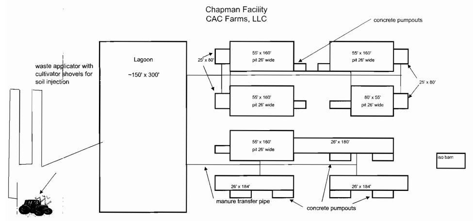
This swine facility utilizes total or partial slatted pits under all buildings. The concrete slats, as well as the 6' deep concrete pits are all a part of the pollution control facility. In addition, these buildings have concrete pumpouts that facilitate timely & accurate waste removal. All pits are also connected via PVC pipe transfer line to the lagoon, which is used as an additional waste control storage when necessary.
